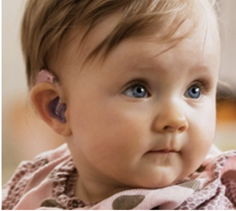
Baby with a BTE hearing aid (sits behind the ear) which is connected to a custom-fit earmold (sits inside the ear).
